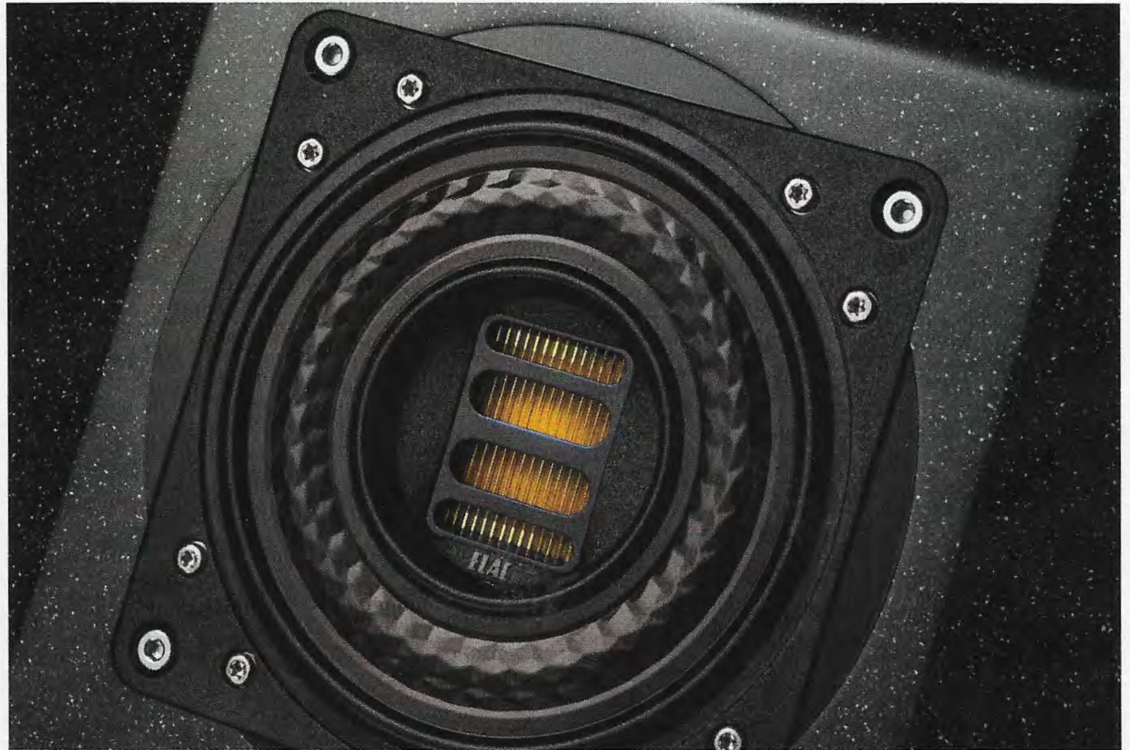
Removing the grille from the mid/high Elac driver reveals its unusual construction. The highs are handled by an AMT tweeter, while the mids are taken care of by a ring-shaped diaphragm around the outside.
